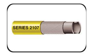
Series 2107 has a specially formulated yellow cover to provide extended abrasion life. This hose will also resist oils, chemicals, animal fats and meets MSHA requirements. Ideal for mines, construction sites, factories, food processing, agriculture and many more applications. RMA Class A tube/cover. Non-conductive.
